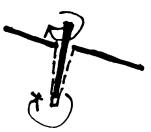
3. Place live pole in hole started by stake. Place a board on top of the pole and then hammer the live pole in. The board protects the pole from splitting.
