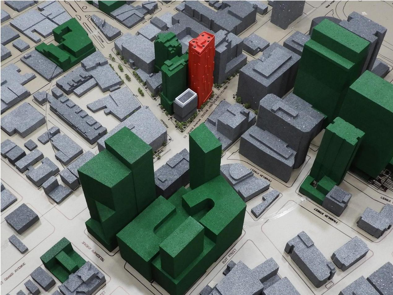
**Image 2E: Wind Tunnel Study Model - Project + Cumulative Configuration**
