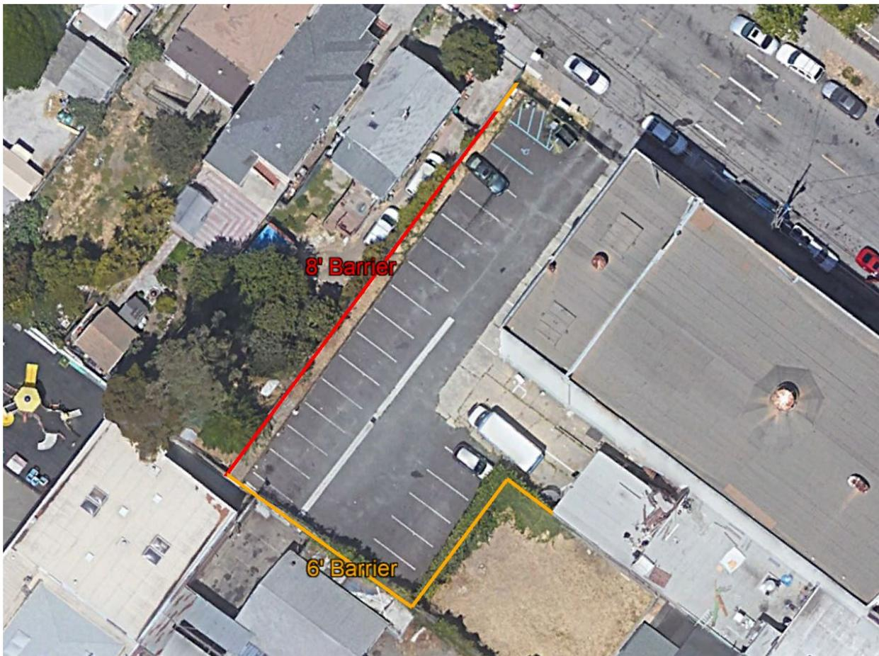
**Figure 15: Existing 6-foot and Proposed 8-foot Noise Barriers**
